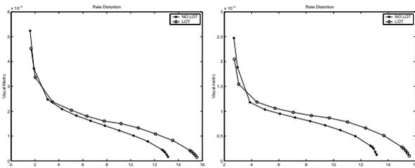
**Fig. 5.** Rate-distortion curves : *venus* (left) and *head* (right) models for compression (optimal basis). Uniform quantization precision was 16 bits. We could not distinguish the reconstructed model from  $D_{vis} = 1.3 \times 10^{-5}$  (*venus*) and  $D_{vis} = 1.4 \times 10^{-4}$  (*head*) on. Overlapping results approximately in a 1 bit/vertex overhead, but provides much better quality at the beginning of the reconstruction.
