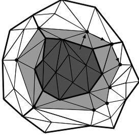
**Fig. 3.** Patch augmentation by overlapping : in this example the mesh is partitioned in 4 patches. The patch being augmented is represented in dark grey. The vertices selected for the overlapping on the neighboring patches are chosen in a spiral way as shown by the arrows. The patch resulting from the augmentation is represented in dark and light gray.
