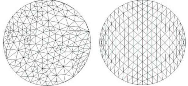
**Fig. 2.** *Left:* A patch after Tutte projection. The vertices are located at the center of their neighbors. The vertices still have original connectivity but they now have 2D-only coordinates. The grid contains 196 vertices. *Right:* Regular grid on which to map the Tutte projected vertices. The grid contains 196 vertices
