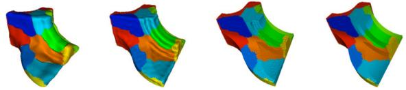
**Fig. 6.** Various stages of on-the-fly mesh geometry decoding. We took 20% overlapping (480 vertices per patch after augmentation). On CAD objects, many coefficients are needed to better reconstruct the geometry.  $D_{vis}^{5\%} = 7.7 \times 10^{-5}$ ,  $D_{vis}^{15\%} = 4.56 \times 10^{-5}$ ,  $D_{vis}^{75\%} = 1.3 \times 10^{-5}$ ,  $D_{vis}^{90\%} = 0.62 \times 10^{-5}$ . The model is well reconstructed from  $D_{vis} = 5 \times 10^{-6}$  on.
