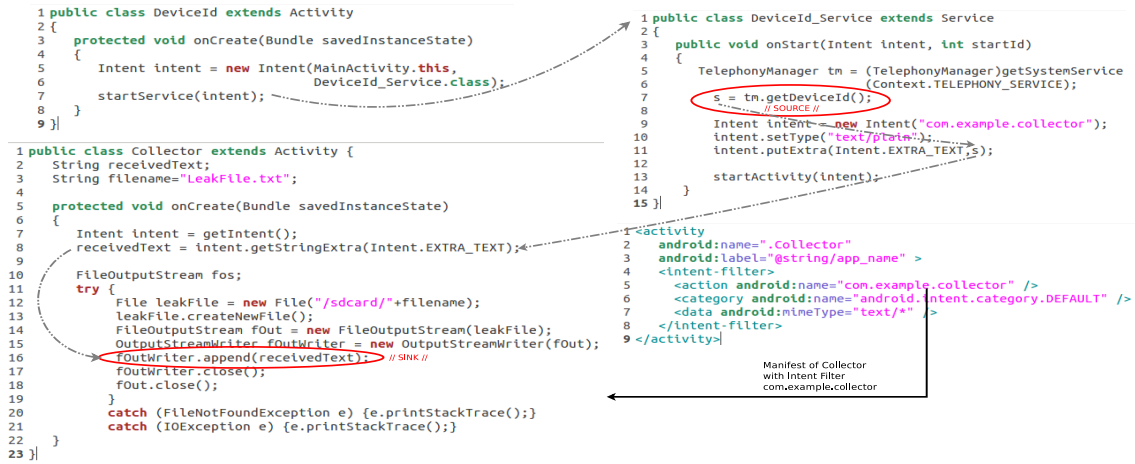
Figure 1: Examples of the privacy leakage path spread across apps DeviceId, DeviceId_Service and Collector
