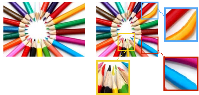
Figure 2: Illustration of local region distortion. Left: the original image of pencil . Right: the retargeted result using the seam carving method in [1] with three zoomed-in local regions.
