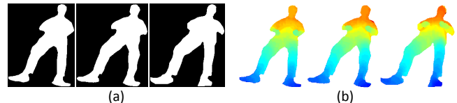
Figure 1: Silhouettes ambiguities in poses. Pose differences (due to different hand positions) cannot be seen from silhouettes in (a), but are readily visible from three-dimensional shape information in (b).
