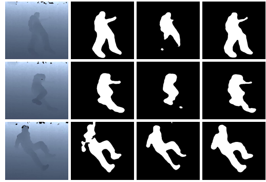
Figure 6: Results of depth image segmentation. First column: Input depth image. Second and third columns: Segmentation mask obtained after applying standard background subtraction method [35] on color and depth images respectively. Fourth column: Segmentation mask obtained by our algorithm.
