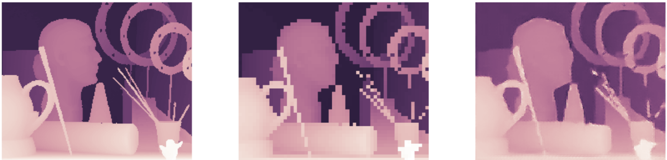
Figure 9: Example of depth super-resolution. Left to right: ground truth, input, \times 8 upsampled output
