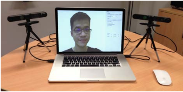
Figure 1: Our robust setup: with only two consumer grade RGBD cameras.
