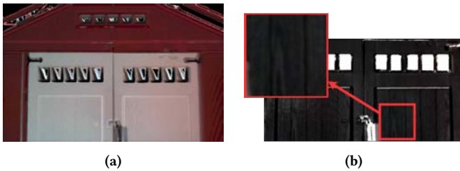
Figure 4: LaFortune BRDF: diffuse map(left), specular map(right). The inset picture in the specular map (b) is a close-up of the region indicated with red and demonstrates the level of detail captured by this approach.
