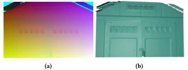
Figure 3: Experiment #1: (a) The XYZ map of the scene’s structure generated with SLS. (b) A render from a novel viewpoint of the reconstructed geometry.
