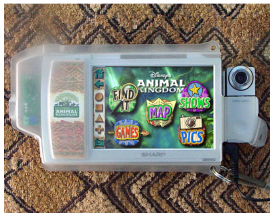
Figure 1: The PDA Showing the “Home Page”. There are five hyper-link buttons on the screen. To the left of the screen there are seven silk-screened buttons. Attached to the right is the digital camera.
