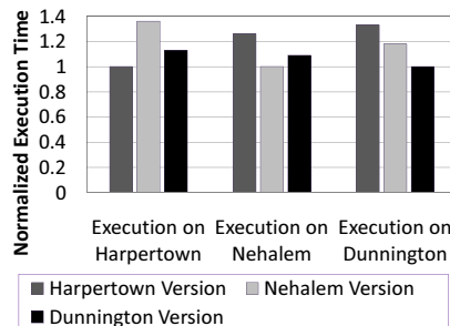
Figure 2. Normalized parallel execution times for a multi-threaded application ( galgel ) on different Intel multicore architectures.
