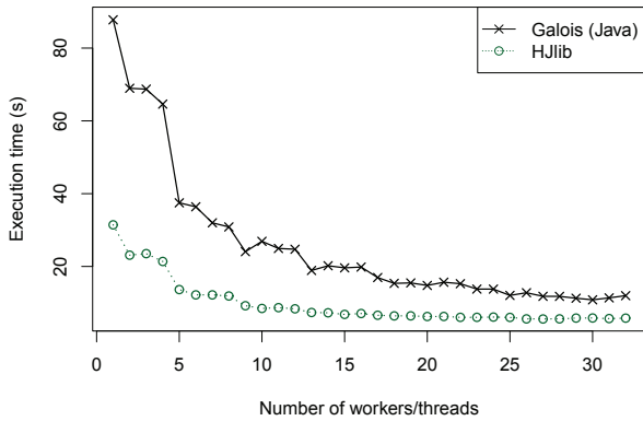
(a) Minimum execution time as a function of number of workers for Galois and HJlib versions
