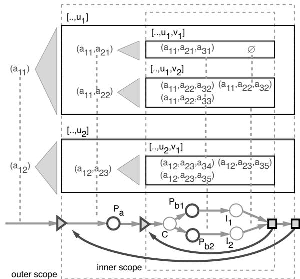
Figure 3: Dataflow-join topology with the Faucet pattern applied.
