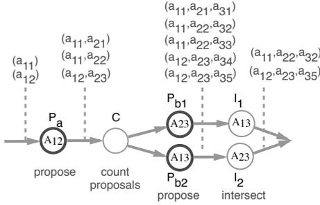
**Figure 1: Logical topology for the dataflow-join computation.**
