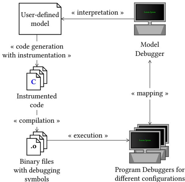
Figure 1: Model-Level Debugging Workflow
