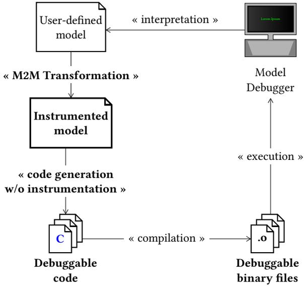
Figure 3: Model-Level Debugging Workflow
