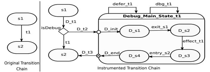
Figure 4: Model Instrumentation Overview
