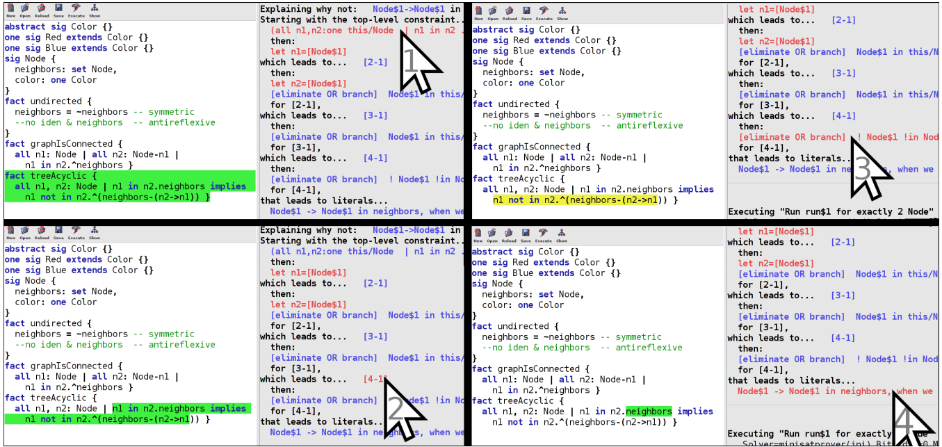
Figure 2: Sample provenance and interaction for the 2-node model in Fig. 1 asking why Node$1 cannot have a self-loop edge. The right-hand side of each of the four panels is a step-by-step deductive argument. The left-hand side highlights portions of the specification corresponding to where the user is pointing in the right-hand pane. Yellow highlights (shown in panel 3) comprise the set of subformulas that force local necessity (Sec. 3). Green highlights (shown in panels 1, 2, and 4) correspond to steps of the recursive descent algorithm we present in Sec. 4.
