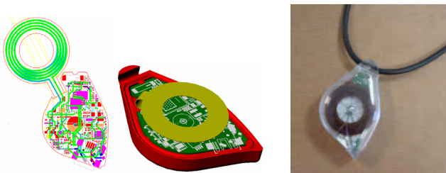
Figure 2 – SOLO, a wearable smart thing. Pendant-like device for personal affinity matching and personal data management. Features: Zigbee and contactless power supply.
