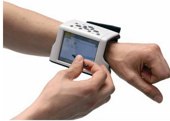
Figure 1 – Zypad, a wrist worn wearable Computer. Main Features: Touch screen, GPS, WiFi, Bluetooth. Optional functions: Zigbee or RFID reader. Operating systems: Linux or Win CE.
