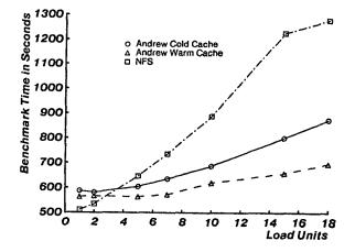
This figure compares the benchmark times of NFS and the Andrew file system as a function of load. The clients were Sun3/50s with 4 Mbytes of real memory and a 70 Mbyte local disk. The server was a Sun3/160 with 8Mbytes of real memory and two 450 Mbyte disks. In the NFS experiments, at loads of 10 or more, some of the clients failed to complete the final phase of the benchmark. Refer to the paper for more details.
