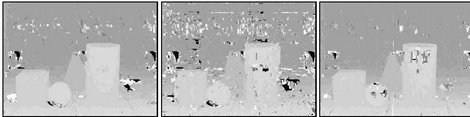
Figure 4. Depth maps obtained for the synthetic scene using simple winner-take-all. Left: computed over a set of images with same exposure using SSD. Middle: computed over a set of images with varying exposure using NCC. Right: computed after converting all images to radiance space and running multi-view stereo with SSD.
