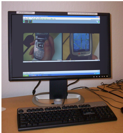
Figure 8: Monitor with live video feed used by moderator to observe the user's screen and keypad
