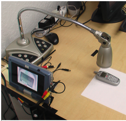
Figure 3: Document camera system with small monitor for moderator to observe the user's screen
