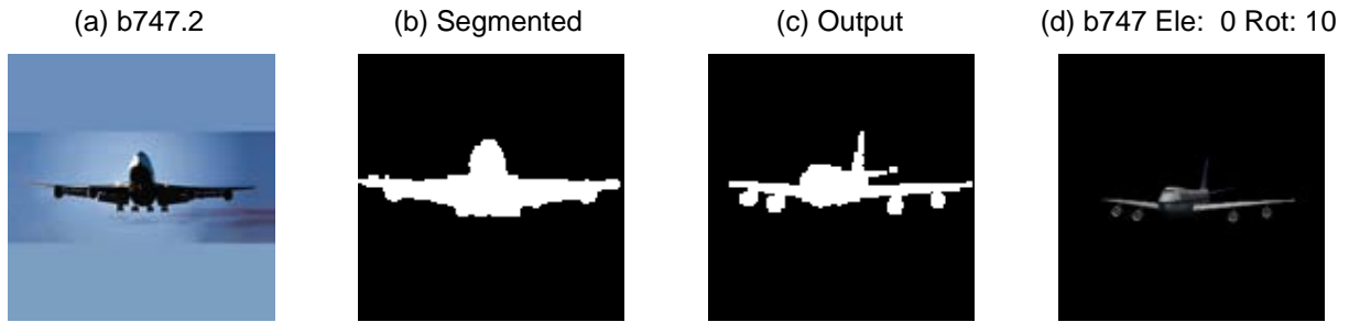
Figure 10. (a) input image, (b) normalized image, (c) image/pose from classifier output, (d) 3-D rendered image based on classifier output.
