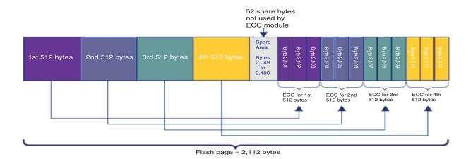
In this configuration the Hamming code requires 3 bytes of ECC information for each 512-bytes sector, or 12 bytes (96 bits) of ECC encoding information is required per 2KB page.
