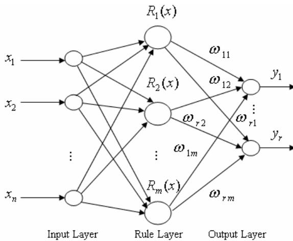
Figure 1. RBF based FNN structure.
