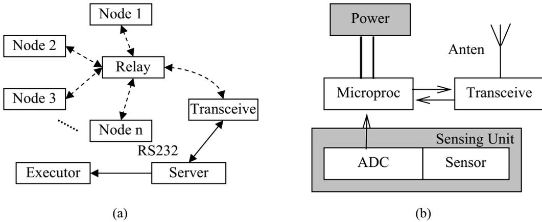
Figure 3. (a) System structure. (b) The components of a sensor node.
