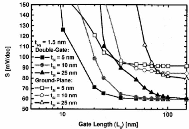
Fig-15: The S-factor for DG MOSFET and for ground plate MOSFET. For DG MOSFET very close to ideal is achievable and for ground plate DIBL is 20-30 mV/dec worse than the double gate. The fixed bottom gate potential results in a capacitor divider, reducing the control of top channel potential by the top gate. Bottom gate insulator for ground plate is 2.25nm thick.
