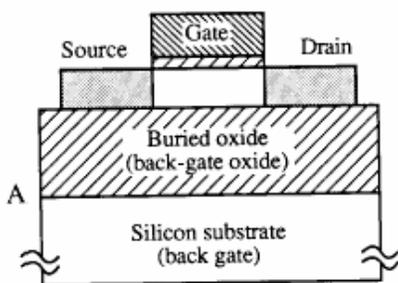
Fig- 5: Conventional thin film SOI MOSFET
