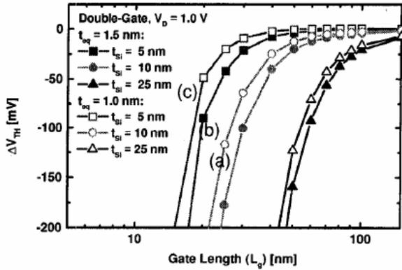
Fig-12: Threshold voltage roll-off for double gate with  $t_{eq} = 1.5$  and  $1.0$  nm.
