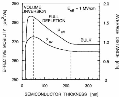
**Fig- 22:** Electron effective mobility in the symmetrical double-gate SOI transistor according to the “classical” and “quantum” models of the semiconductor region and the local mobility model.
