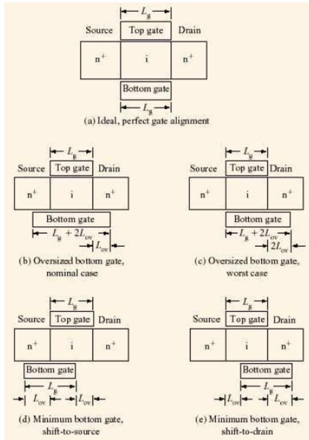
Fig- 16: Cases of misalignment in DG MOSFETs
