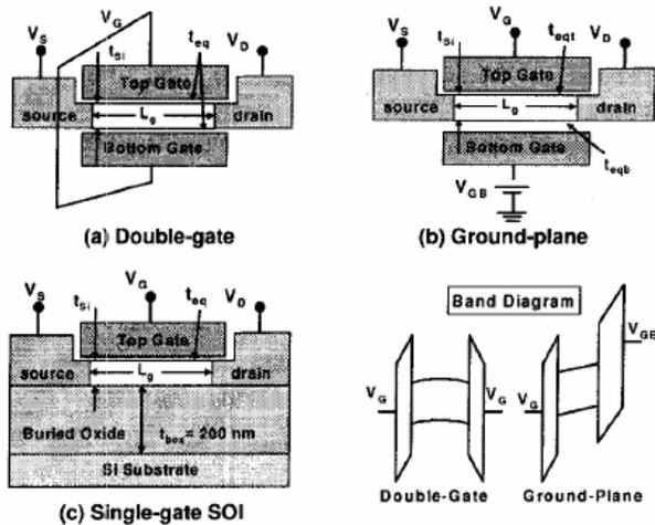
**Fig- 11:** Double gate, (b) ground plate, (c) single-gated SOI MOSFET. Gate work function is set at mid-gap of the silicon film band gap. On chip biasing of the ground plate is assumed. The source/drain junction is abrupt. The channel length is the metallurgical channel length.
