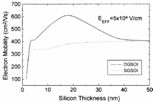
**Fig-19:** Evolution of electron mobility for a DGSOI (solid line) and a SGSOI (dashed line) with the thicknesses of the silicon layer. All the scattering mechanisms were taken into account.
