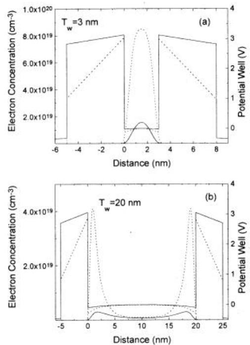
Fig-17: Electron distributions for different thicknesses of the silicon slab in a DGSOI structure. Two different effective electric field values were considered [7]
