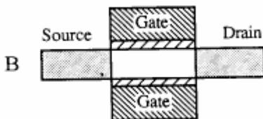
Fig- 6: SOI MOSFET with top and bottom gate
