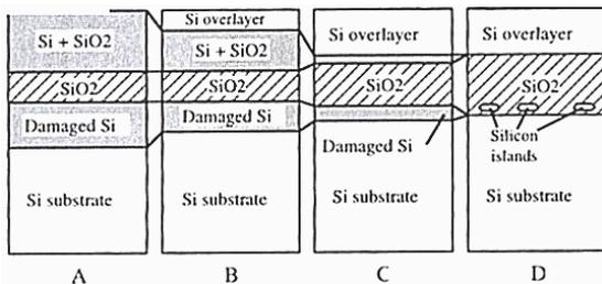
**Fig-3:** Evolution of the structure of the SIMOX structure as a function of post-annealing temperature (implant dose=  $1.5 \times 10^{18}$   $\text{cm}^{-2}$ , energy = 200 keV). A) as implanted, B) 2-hr. annealing at 1150°C, C) 6 hour annealing at 1185°C, D) 6 Hr. annealing at 1300°C.
