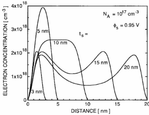
**Fig- 21:** Influence of the semiconductor thickness on the electron concentration distribution at the surface potential constant, according to the “quantum” model.
