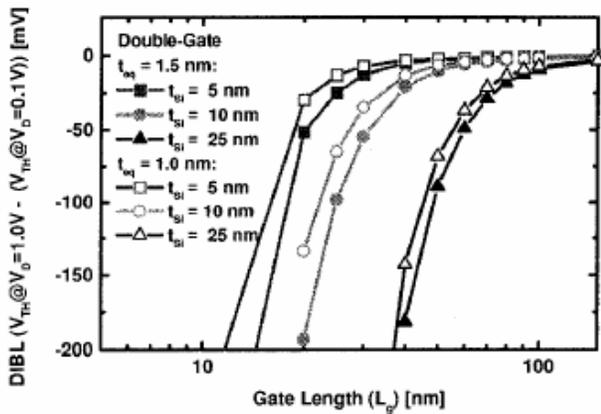
Fig-13: DIBL for double gate with  $t_{eq} = 1.5$  and  $1.0$  nm.
