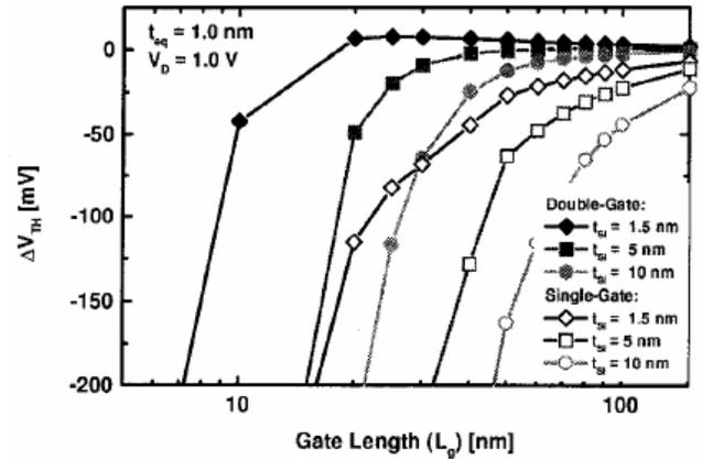
Fig-14: Threshold voltage roll-off for double gate and single gate MOSFET. Single gate will not meet the short channel effect requirements.
