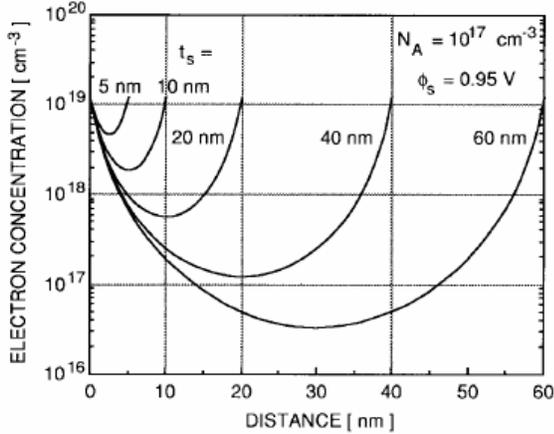
**Fig-20:** Influence of the semiconductor thickness on the electron concentration distribution at the surface potential constant according to the “classical” model.
