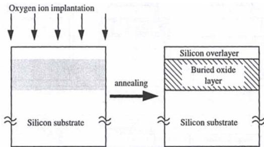
**Fig-2:** The principal of SIMOX: a heavy dose oxygen implantation into silicon followed by an annealing step produces a buried layer of silicon dioxide below a thin single crystal silicon overlayer.
