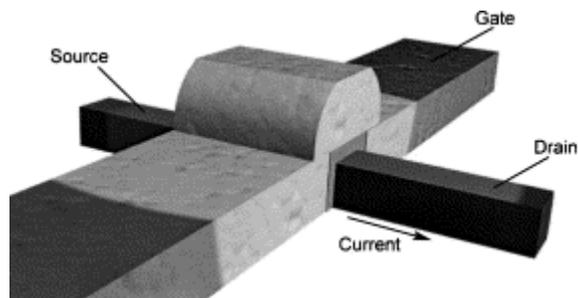
Fig- 9: Triple-gate SOI MOSFET.
