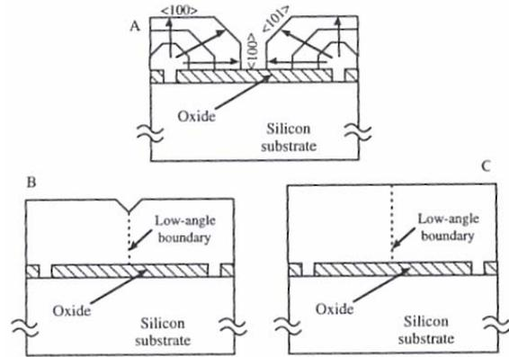
**Fig-1:** ELO technique. A) growth from seeding window, B) coalescence of adjacent crystals, C) self-planarization of the surface.
