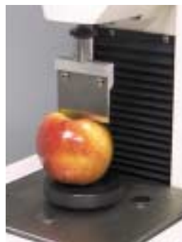
Sample fixtures for analyzing food texture
