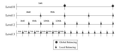
Figure 5: Integrated Execution Order showing Points of Load Balancing
