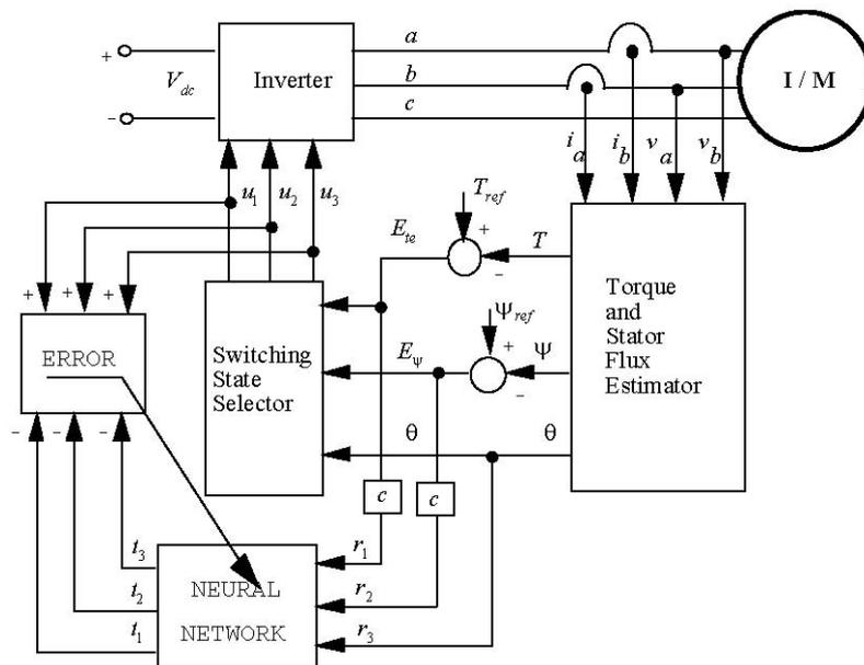
Figure 3 Schematic of DTC using Neural-Network controller
