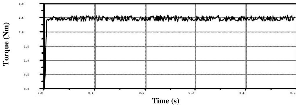
Figure 13 Torque developed in DTC using neural network trained with genetic algorithm (Binary coding representation)
