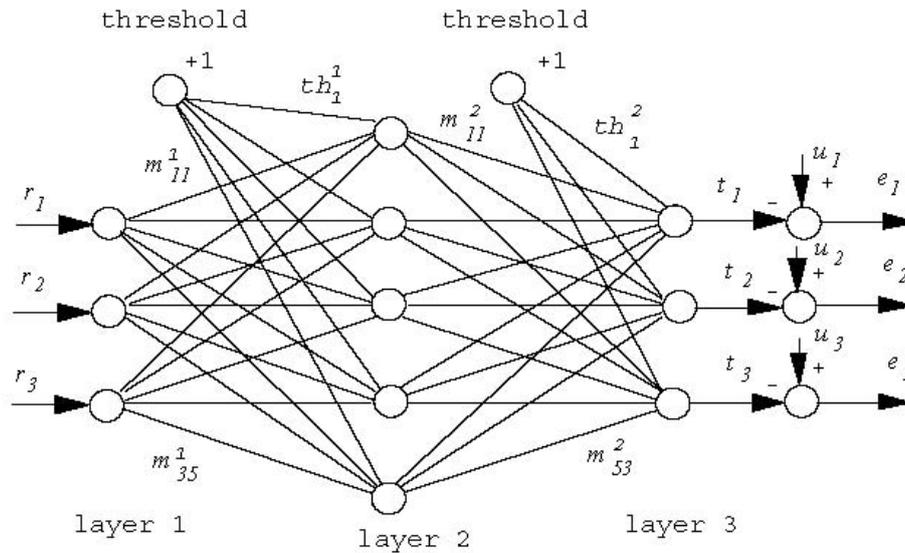
Figure 8 Structure of neural networks trained using GA
