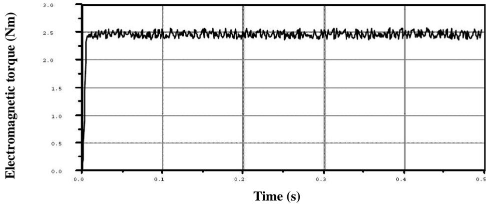
Figure 12 Torque developed in DTC using neural network
