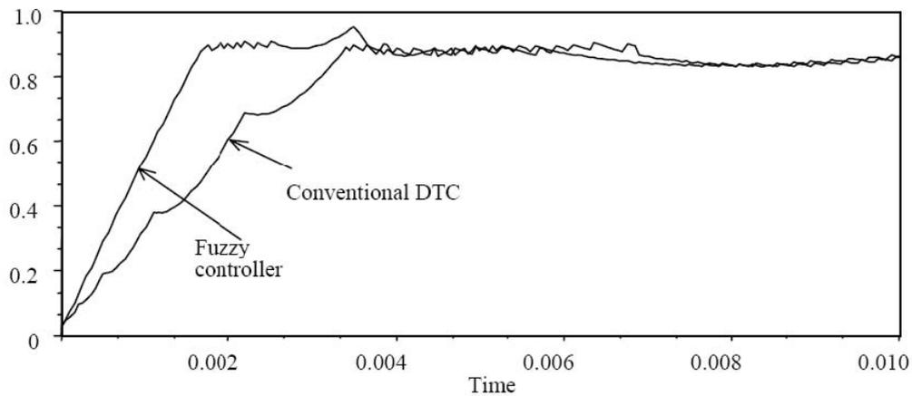
**Figure 19** Initial stator flux rise
