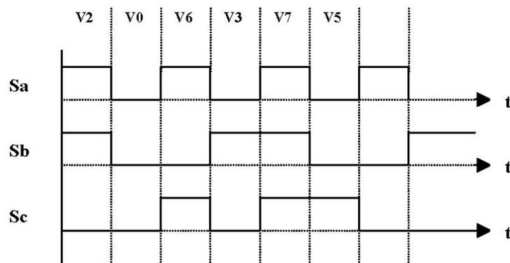
**Figure 2** Generation of Pulses for PWM inverter when flux vector lies on sector 1
