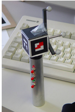
(a) The light saber used as an input-device by the user with attached markers valid for both systems.
