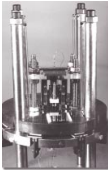
Pictured: A scanning tunneling microscope, made in the Nanoelectronics Laboratory by Prof. Chia-Hung Yang's research group. This type of microscope resolves down to the atomic level, enabling Yang's group to probe the quantum nature of devices at the nanometer scale.
