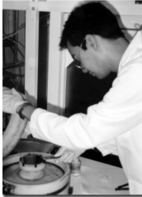
Pictured: (left) Student Marcel Pruessner applies an adhesion promoter to a silicon wafer, which will have resist spun on it, in the new Integrated Circuits Fabrication Course. The facility used in this course is housed in the Institute for Plasma Research.
