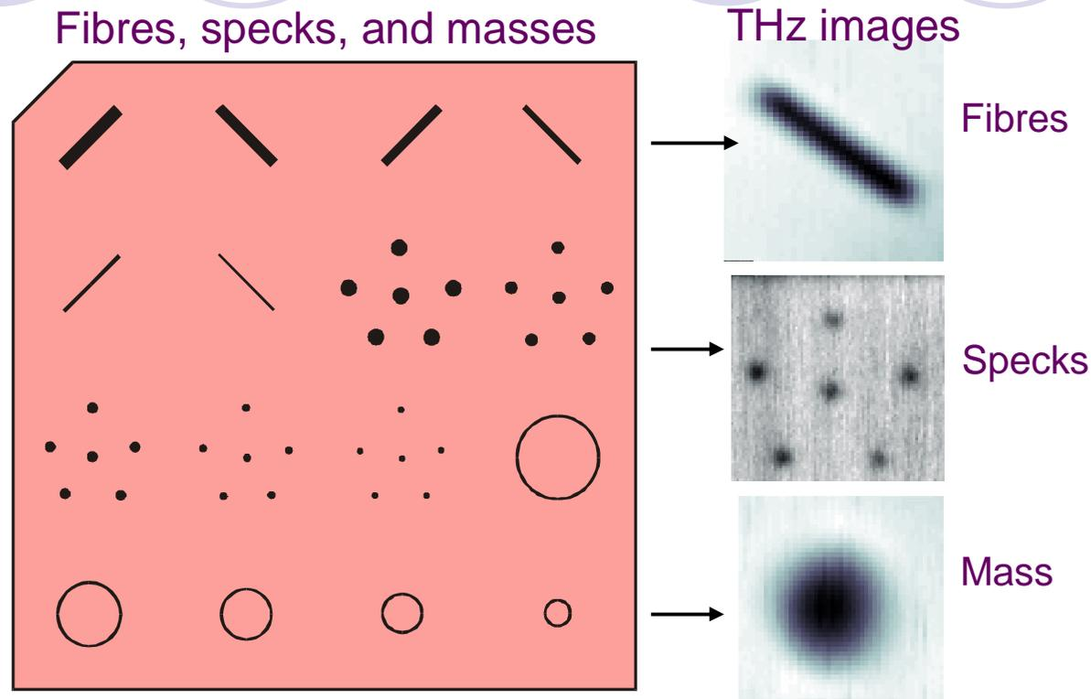
Phantom is designed to perform a quantitative evaluation of the system's ability to image small structures similar to those found clinically. THz system resolved **0.4 mm fibre**, **0.25 mm mass** and **0.24 mm speck**.
