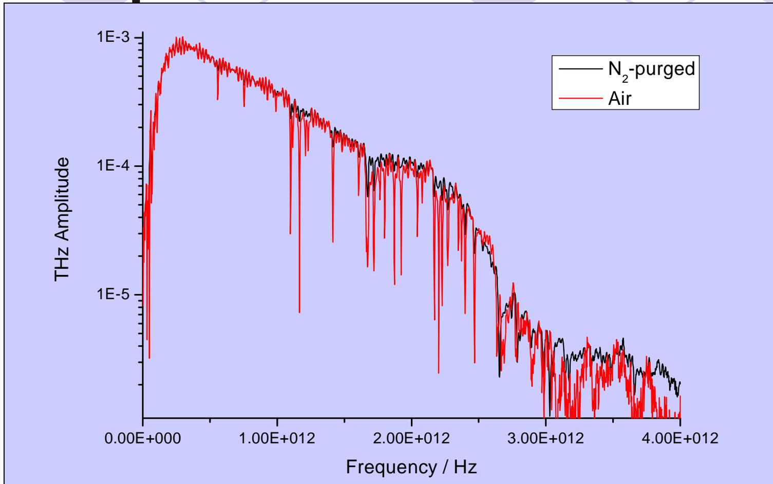
Bandwidth dictated laser pulse duration, electro-optic detection material, etc.
