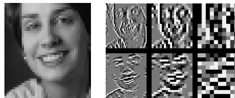
Fig. 2. Representing a candidate face image for face detection. Given an image (left), a discrete wavelet transform is computed and quantized (right); we keep the HL and LH bands at 3 scales. Each feature used for detection is a combination of 4 quantized DWT coefficients.
