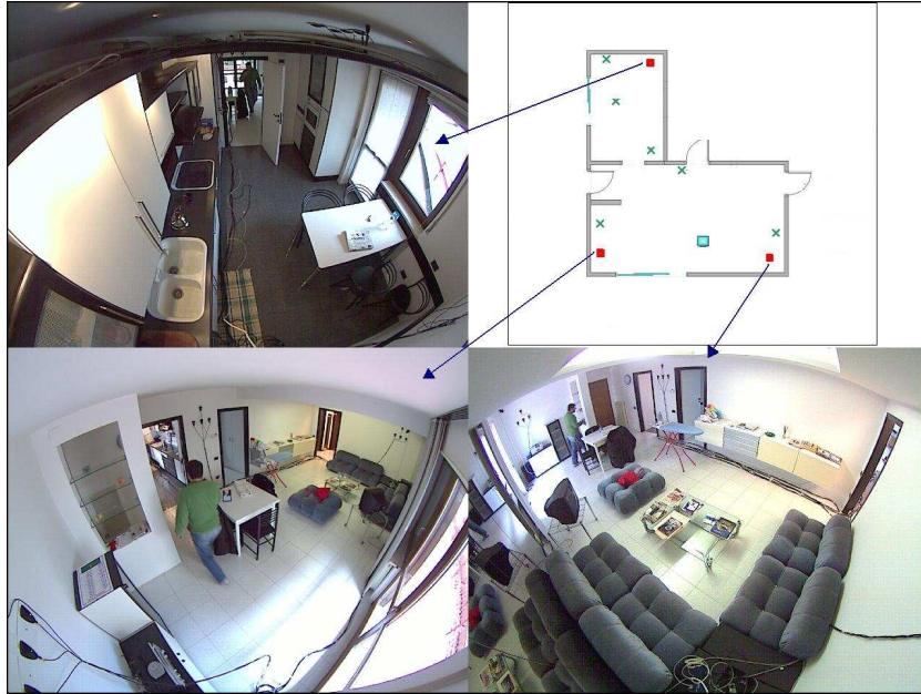
Fig. 1. A schematic diagram of the smart home used in the ADL corpus collection [8], depicting the audio-visual sensor locations (upper right). Example views of the three cameras are also shown.
