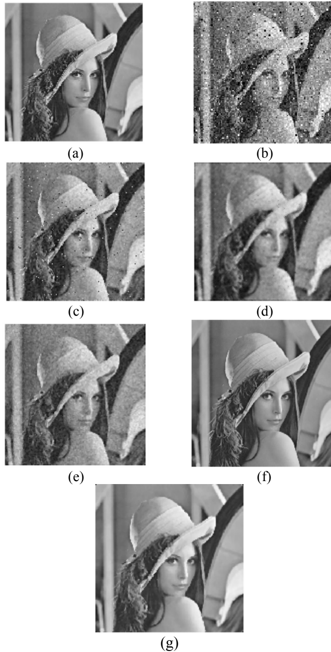
Figure 4: (a) Original Lena image, (b) Lena image corrupted by Gaussian and Salt & Pepper noise, (c) Normal wiener filtering result, (d) Improved adaptive wiener filtering result, (e) Median filtering result, (f) Noise filtering result, (g) Result of the novel Hybrid filter.
