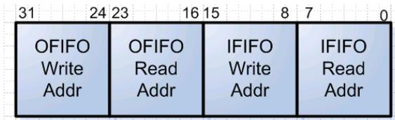
Figure 3.18: FIFO Address Register
