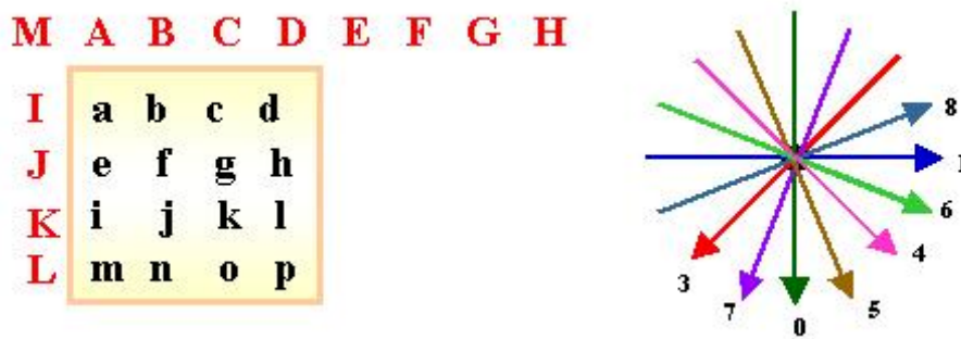
Figure 3. Intra prediction modes for 4x4 luminance blocks.
