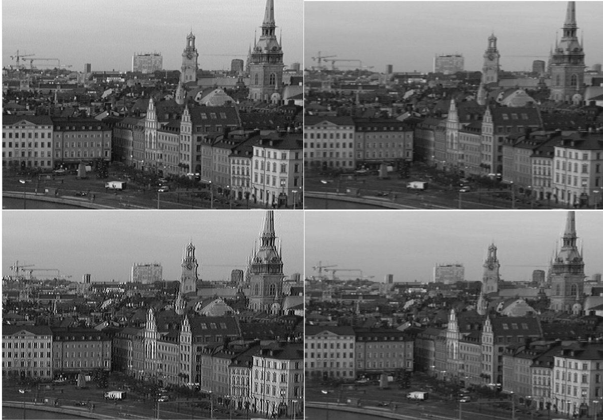
Figure 7: Stockholm scene before and after processing. Top-Left: Original Image. Top-Right: Simulated Motion Blur. Bottom-Left: Preprocessed Image. Bottom-Right: Simulated Perceived Image
