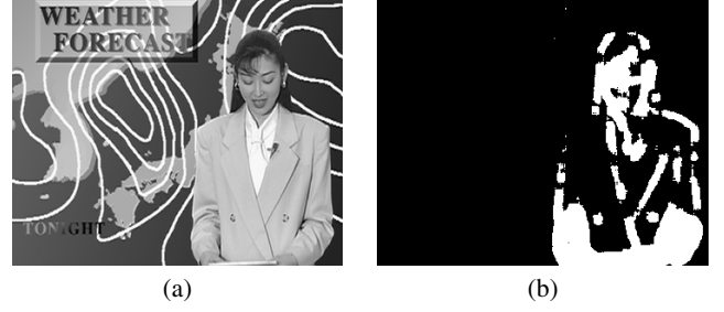
Fig. 2. (a) Sequence Weather . (b) The moving pixel mask mp(x, y, t) .
