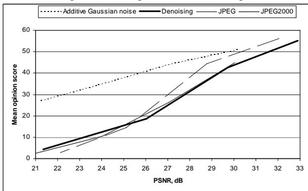
Fig 5. Dependence of the opinion score on PSNR for some types of distortions
