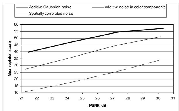
Fig. 6. Dependences of the MOS on PSNR for different spatial frequency and color distributions of additive noise
