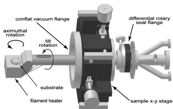
FIG. 7. Schematics of GLAD manipulator. The azimuthal and tilt rotations are executed by two stepper motors (not shown). To scale.
