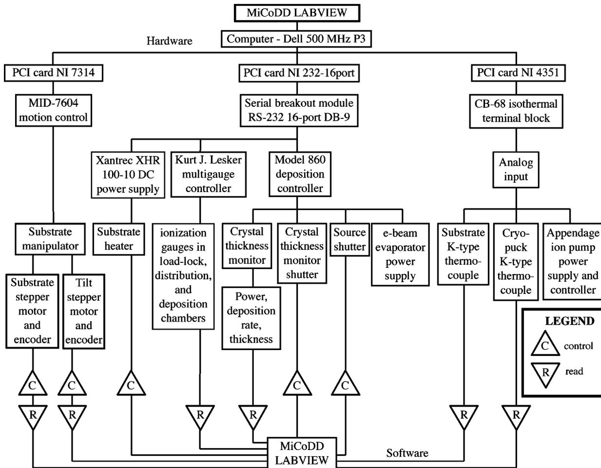
FIG. 8. Schematic diagram of communication interface for the LabVIEW deposition program.
