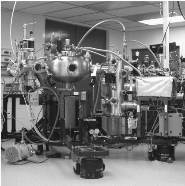
FIG. 3. Photograph of the GLAD UHV deposition system.
