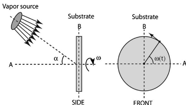
FIG. 2. Schematic description of the GLAD process. Angles of substrate tilt  $\alpha$  and rotation  $\omega(t) = \text{const}$  are controlled by stepper motors situated outside the vacuum system operating through a feedthrough and gear system.
