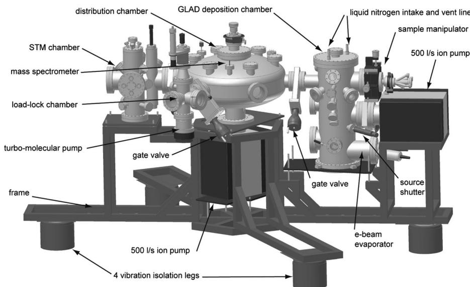
FIG. 4. Three-dimensional layout of the GLAD UHV deposition system. To scale.
