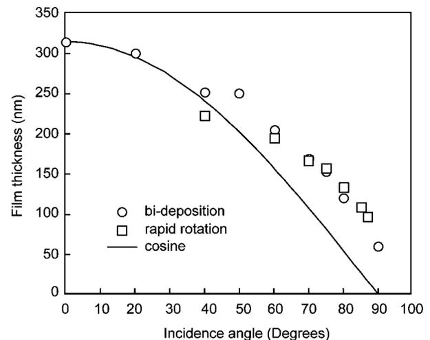
FIG. 9. Calibration of the film thickness profile—film thickness versus incidence angle.
