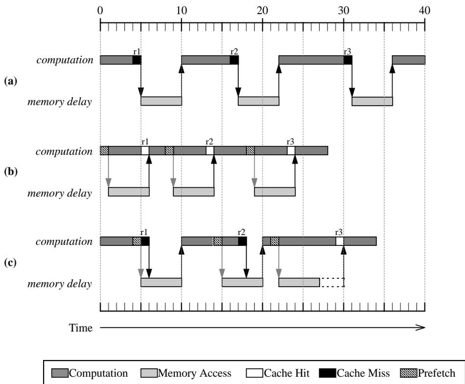
**Figure 2.** Execution diagram assuming (a) no prefetching, (b) perfect prefetching, and (c) degraded prefetching.
