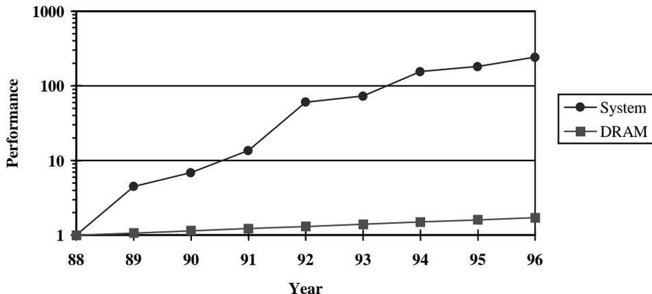
**Figure 1.** System and DRAM performance since 1988. System performance is measured by SPECfp92 and DRAM performance by row access times. All values are normalized to their 1988 equivalents (Source: Internet SPECTable, <ftp://ftp.cs.toronto.edu/pub/jdd/spectable>).
