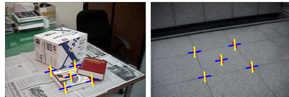
Figure 1. labelEstimateCoord2Estimating the direction of Z-axis by rotating the image coordinates
