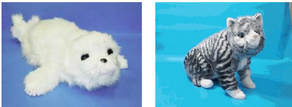
Figure 1.5. The Paro seal robot (left) and the Tama cat robot (right) developed for therapeutic use.
