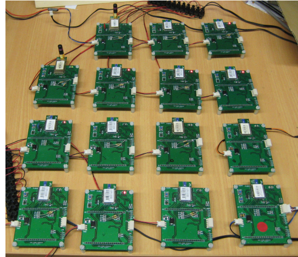
Fig. 1: Our 15-node ZigBee-based communication system.
