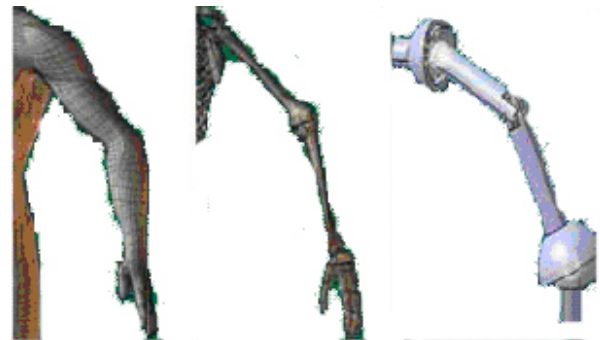
Fig. 2. Configuration of human upper limb and its equivalent mechanical model
