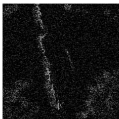
Figure 19. Variance for Daubechies Wavelet for Long Crack & Blob defect tile image
