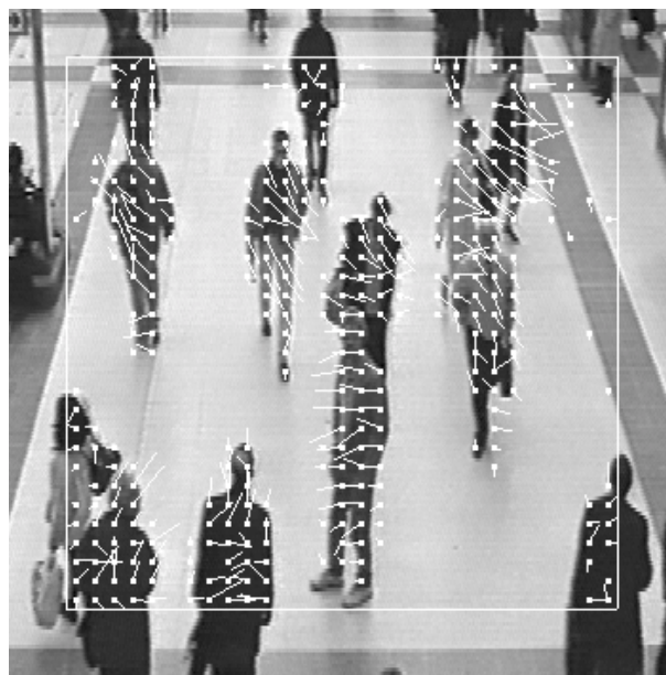
Fig. 14: A typical result after calculating motion by “block matching”. The white “needles” superimposed on the image represent average magnitude and direction of motion.
