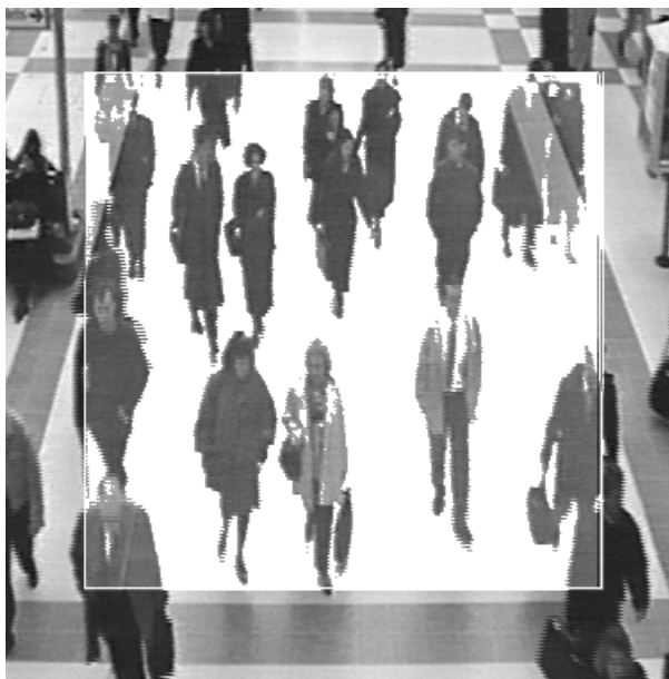
Fig. 6: An image where the background has been removed. The number of remaining “picture elements” has been found to be correlated to the number of people in the image (see Fig. 7)
