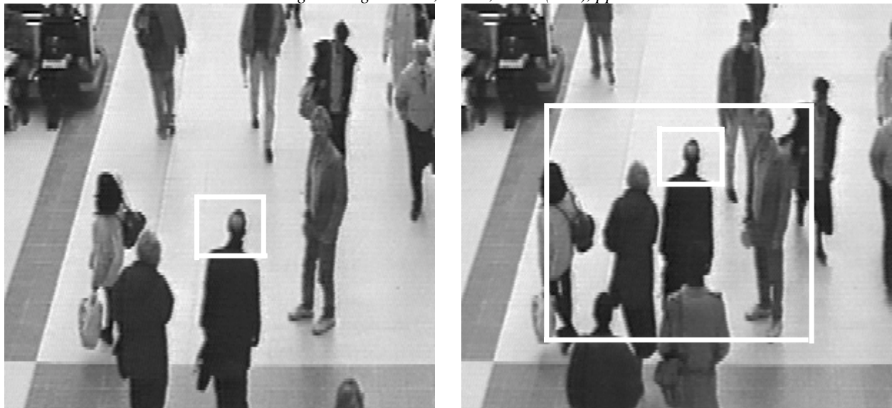
Fig. 13: Motion calculation by “block matching”. A small block is selected as shown on the left image. A “search area” is selected in the next image (on the right) within which a similar block is found. The displacement of the small block between the two images defines a motion vector (see Fig. 14)
