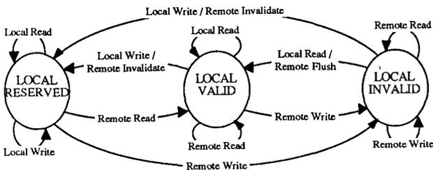
Figure 8: Cluster Adapter State Diagram for Extended Goodman Caching Algorithm
