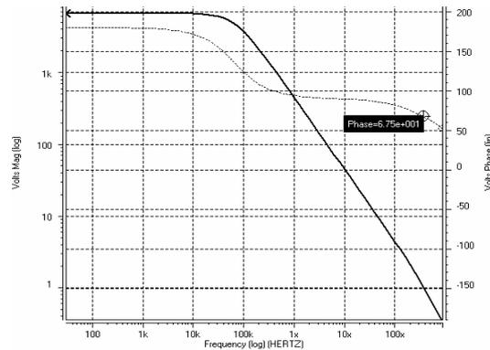
Figure 3. Frequency response of the proposed op-amp
