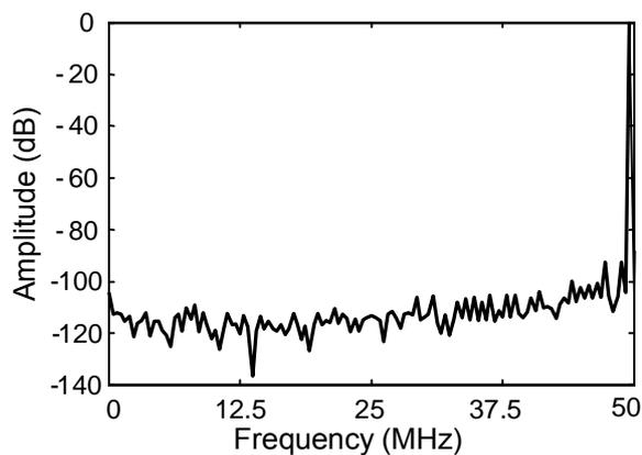
Figure 5. Simulated output spectrum with a Nyquist-frequency full-swing input
