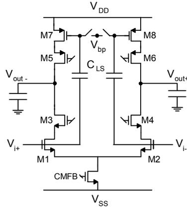
Figure 2. The proposed telescopic-cascode class-AB op-amp schematic
