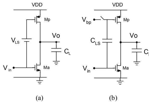
Figure 1. (a) The general schematic, (b) a possible implementation of the proposed switched-capacitor class-AB stage
