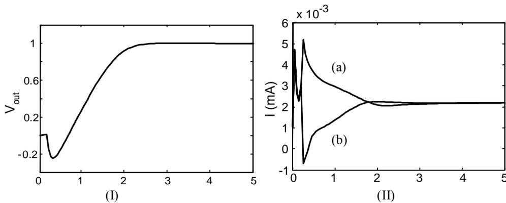
Figure 4. (I) Simulated step response of the SHA, (II) Current consumption while settling, (a)&(b) in  $M8$  and  $M7$  pMOS transistors.
