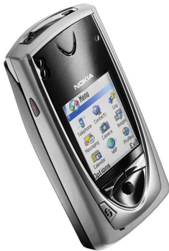
Figure 1. The Nokia 7650. The keypad can be slid out from behind the display, revealing the camera lens on the back
