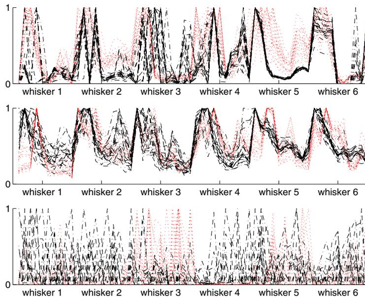
**Fig. 2.** Cumulated feature vectors of twenty sweeps in one position of texture 1 and texture 4. The dotted line indicates texture 1, dashed line texture 4. The preprocessing used was **Top row:** Smoothed raw data, **middle row:** fft and **bottom row:** PCA components after a spectrotemporal analysis.
