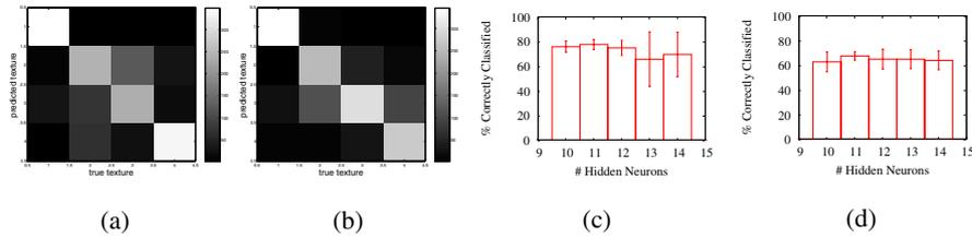
**Fig. 4.** Left Sample hit matrix on all recorded positions and textures with **a)** FFT preprocessing and **b)** smoothed raw data. The textures are from 1 to 4: smooth metal, sandpaper 400, sandpaper 80 and cardboard. **Right** Mean percentage of correctly classified test samples recorded with a mobile robot. **c)** Left whisker array and **d)** right whisker array. The textures to be discriminated were smooth metal vs. rough carton.
