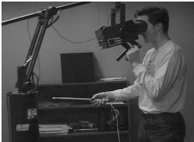
Figure 2: Using the drumstick prop in an immersive virtual environment.
