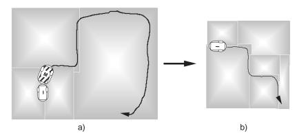
Figure 6: In its most elaborated case, not only movement patterns, but strategies which improve the fitness of the imitator which is running the 'Huegellandschaft' might be learnt. a) The imitator I follows the model M which runs in valleys. Robot I recognizes by means of self-observation, using information from its inclination sensors and batteries that the movements performed by the model are energy-saving. b) Robot I from now on can use the energy-saving strategy of moving in valleys.
