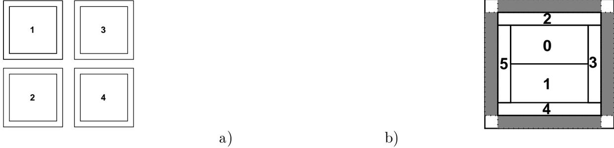
Figure 3: (a) Collective-level partitioning over 4 nodes showing the halo region, and (b) the node-level partitioning on dual-processor nodes, detailing the irregular partitioning used to implement a pre-fetching strategy. The regions marked 0 and 1 correspond to the FloorPlan  $F_i$  in the code of Fig. 8, and the regions marked 2 through 5 to FloorPlan  $F_a$ . This decomposition is duplicated on each node.
